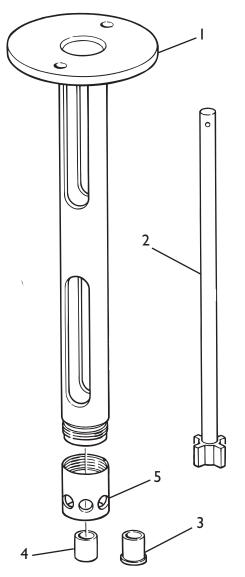
Fig. 17 Replacing the Bushing of the 1, 3/4 & 5/8
