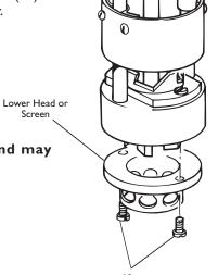
Fig. 13 Changing the Lower Stator - Duplex
