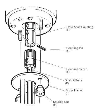
Fig.2 Fitting the Standard Mixing Assembly
