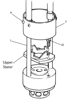
Fig. 14 Changing the Upper Stator - Duplex
