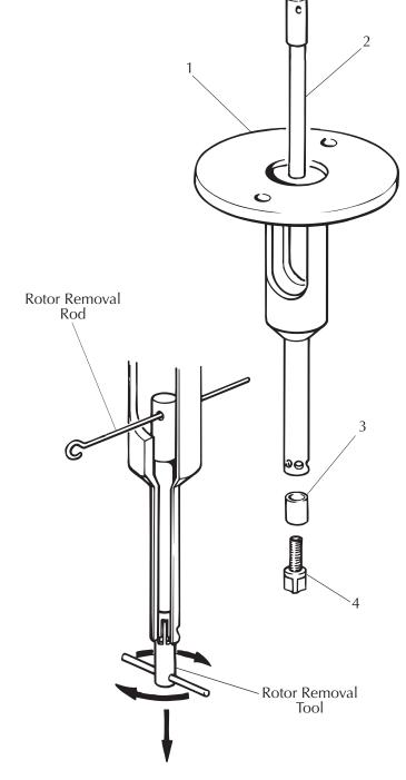
Fig. 18 Replacing the Bushing of the 3/8 Mini-Micro Tubular Mixing Assembly
