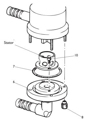
Fig.15 Changing the Head/Screen Laboratory In-Line Mixing Assembly
