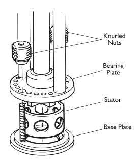
Fig. 10 Changing the Stator
