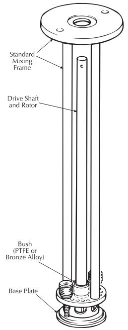
FIG.4 Standard Mixing Assembly
