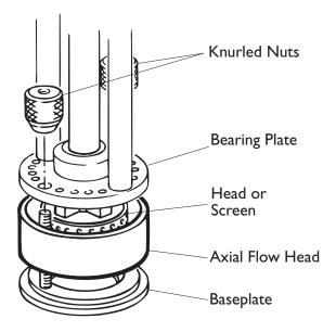
Fig. I I Fitting the Axial Flow Head
