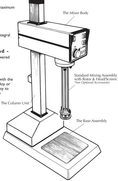
Fig.3 The L4R, L4RT & L4RT-A Mixer Assembly
