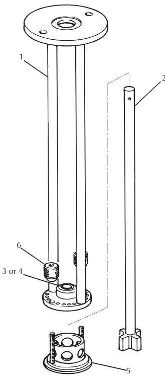
Fig. 16 Replacing the Bushing of the Standard Mixing Assembly
