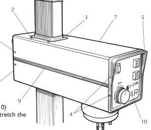
Fig.22 Gaining Access to the Mixer Body
