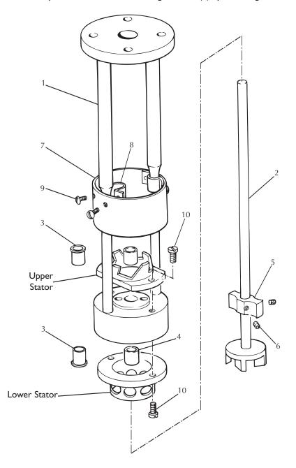
Fig. 19 Replacing the Bushing of the Duplex Mixing Assembly
